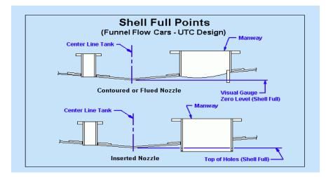
During the time that the tank car tank is being filled with water using the metering or water gauge method, the tank car tank volume can be determined by taking measurements at increasing levels while filling the tank car tank to the maximum level, or what is known as the "shell full" capacity. The metering method uses a calibrated electronic meter to measure the amount of water filling the tank. The water gauge method uses overhead calibrated tanks with
