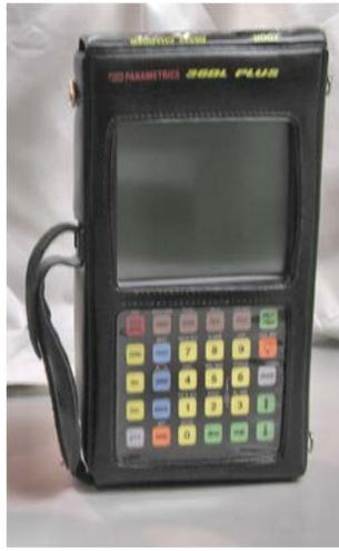
Ultrasonic Thickness Testing (UTT) Ultrasonic Thickness Testing is used to calibrate to a known thickness of any material and the ability to check the thickness anywhere on the component. This technique is used extensively for checking the remaining thickness of the tank car tank shell.
